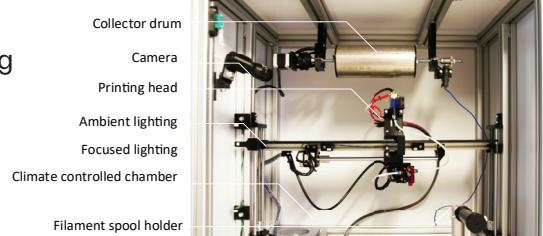
**Polymer melt (FDM filament based) electrospinning setup**
